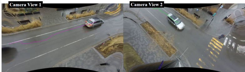
b) Trajectories of the same vehicle through multiple cameras (displayed on the video frames after the correction for lens
