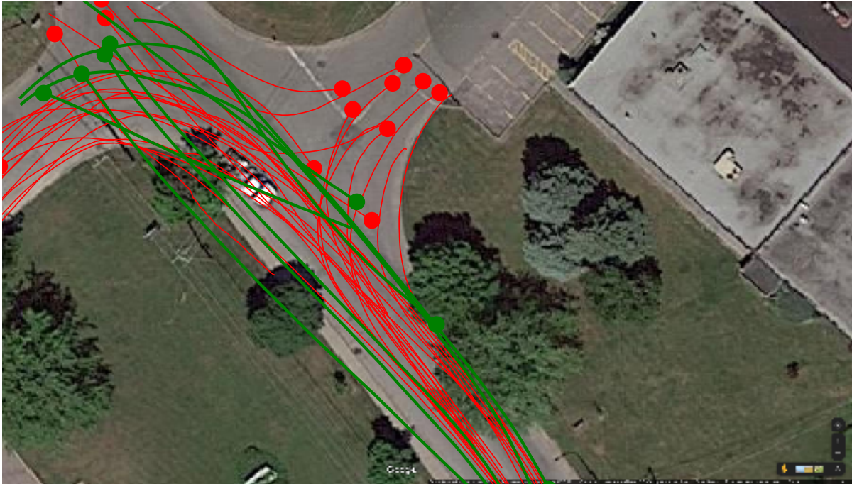
FIGURE 2 Cluster prototypes associated AVs (in green) and other users (in red) at the Mont-calm & Inverness site (origins marked with a circle).
