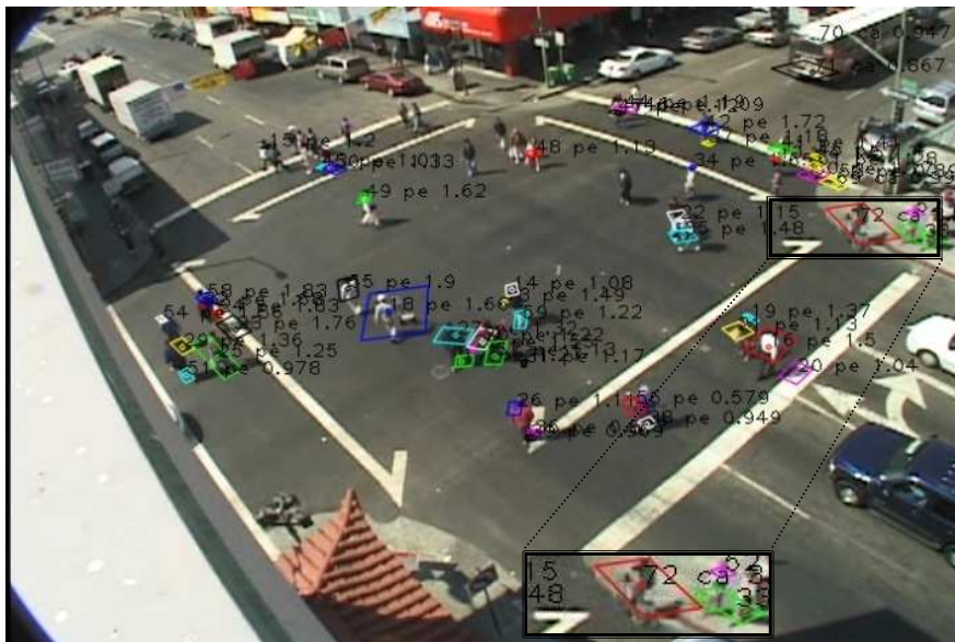
FIGURE 4 Sample frames from validation results. The number of missed detections is 3/32 with 29 false detections mainly due to over-segmentation. Figure a) shows a sample frame from a post-scramble sequence with labeled pedestrians. Figure b) shows the pedestrians tracked in the same frame using the optimized tracking parameters. The bicyclist annotated with a box in Figure b) is correctly identified as a non-pedestrian (given a screen label ‘ca’).
