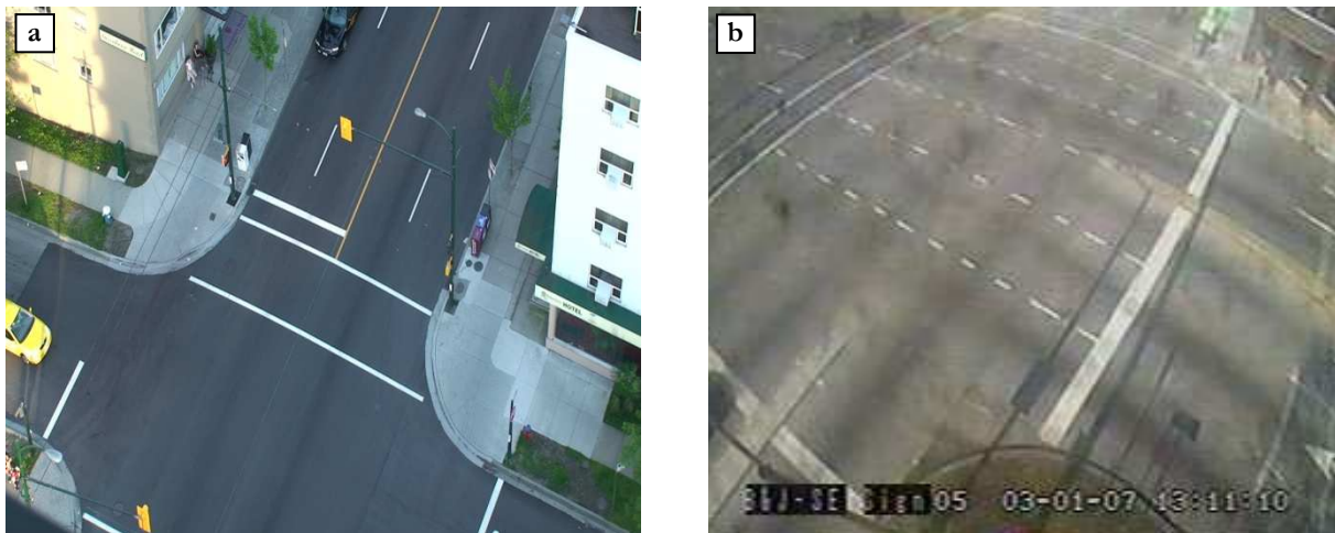
Figure 2 An illustration of camera calibration issues that arise in urban traffic scenes. Figure a ) shows a frame taken from video sequence BR-1 shot at Vancouver-British Columbia. The estimation of the vanishing point location based on lane marking was unreliable. The obtained camera parameters were initially not sufficient to measure pedestrian walking speed in adequate accuracy. The integration of additional geometric constraints enhanced the estimates of the camera parameters and met the objectives of this application. Figure b ) shows a sample frame from video sequence K1 of traffic conflicts shot in Kentucky. Significant radial lens distortion is observed at the peripheries of the camera field of view. A reliable estimation of the vanishing point location requires the consideration of line segments that extend to the peripheries of the camera field of view. The curvature of parallel lines was significant in these locations and the estimation of the vanishing point was challenging.
