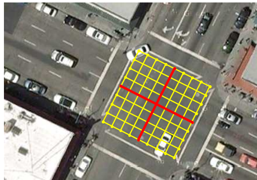
Figure 6 Reference grid for video sequences BR-2, PG, and OK, overlaid over frames of the video sequence and orthographic images. The grid spacing is 1 m and the height of the vertical reference lines (depicted in blue) is 4.0 m. Sequences BR-1 and BR-3:4 are recorded at the same site (BR) with different field of views. Their results grid are similar to BR-2 and omitted for space limitation.
