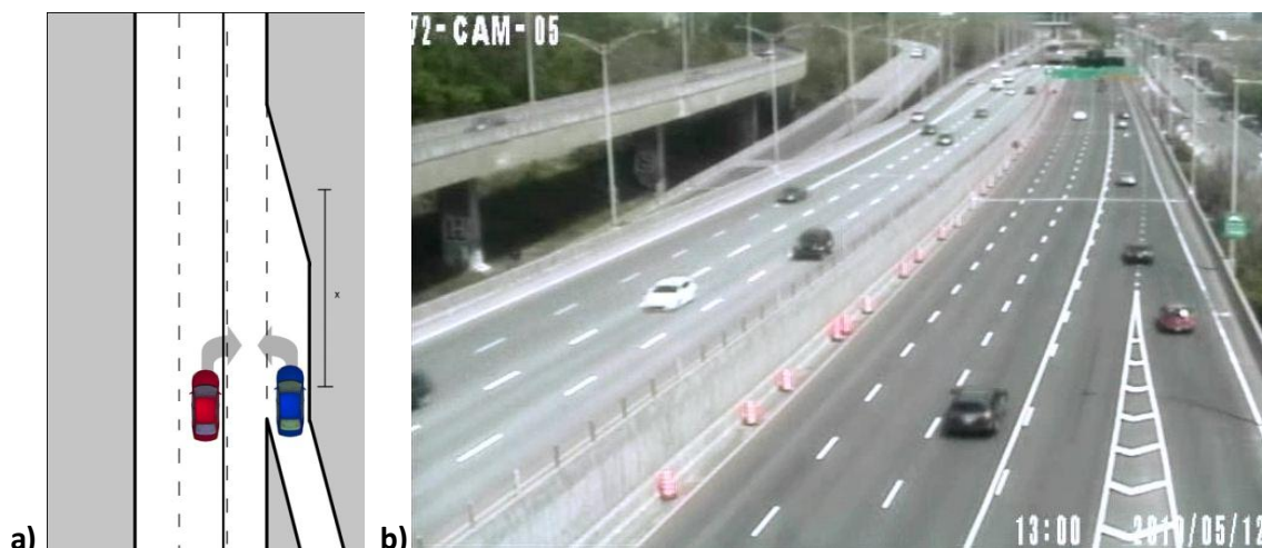
Figure 4: Example LCGV1. a) Exit ramp section diagram demonstrating an LCGV1 and an illegal lane change. Lanes are numbered sequentially starting with the outer-most lane, excluding merging lanes. b) LCGV1 along Autoroute 720 eastbound, entrance 3 (right), Montreal. Source: MTQ.
